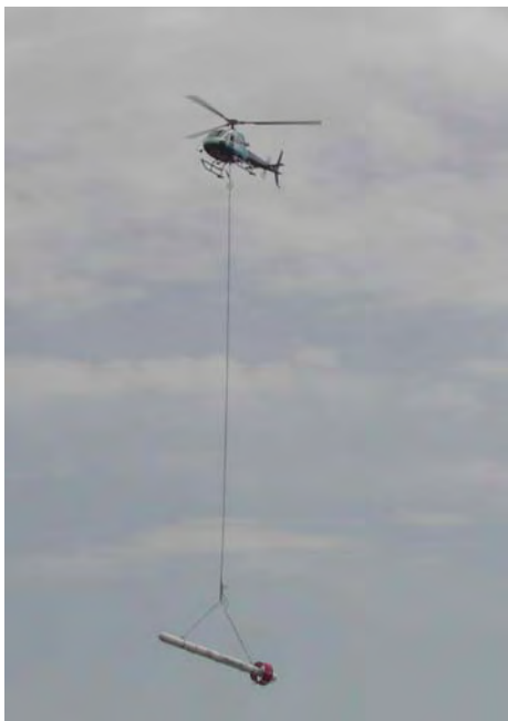
Helicopter and geophysical system. The “bird” is nearly 30 ft long.
