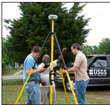
(A) Joseph Zume (OWRB) taking notes as he walks with the backpack-mounted magnetic and GPS system in the western Hunton Anticline. (B) Dan Scheirer (USGS), Joseph Zume, and Carlos Uribe (OWRB) configuring the GPS base station.
