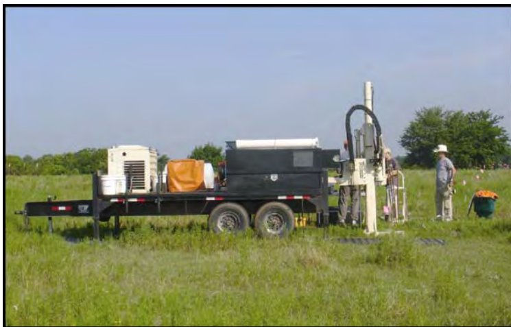
OSU students preparing to collect EC log data for the Arbuckle-Simpson aquifer using the Geoprobe®.
