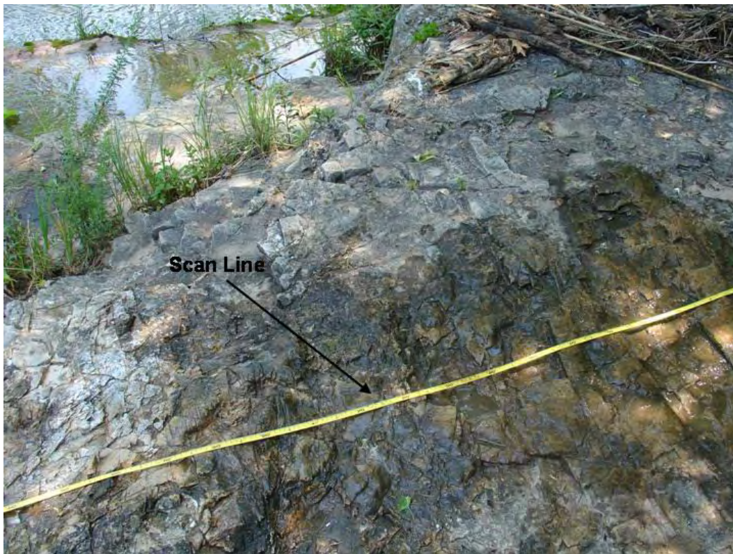
Figure 5. A scan line taken across fractures was used to gather data. One dominant trend is seen perpendicular to the scan line. A second fracture set can be seen parallel to the tape and has grass growing in one of the fractures in the set.
