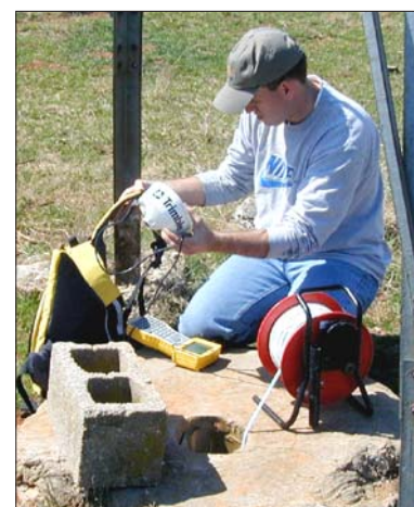
Chris Neel sets up a GPS unit after measuring depth to water in an unused Arbuckle windmill.
