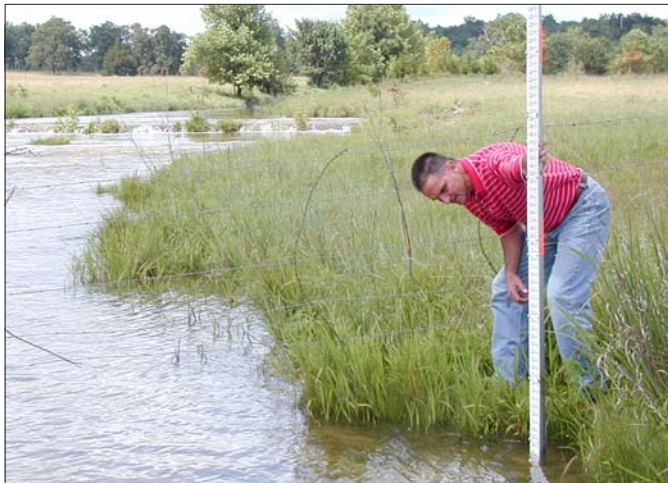
Kelly Self, OWRB environmental specialist, obtains streamwater flow and river stage measurements at Delaware Creek. Weekly discharge measurements are conducted by Board staff at 13 sites throughout the study area.
