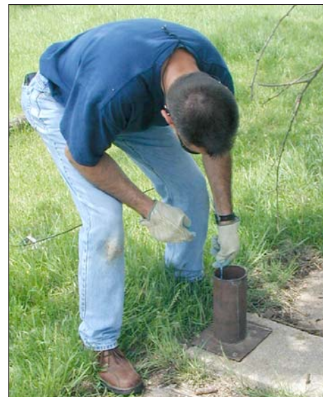
An OWRB hydrologist measures the initial depth of a well selected for installation of a water level recorder. The well, located south of Connerville in the eastern region of the study area, is one of 10 wells equipped with the automated groundwater level recording device.
