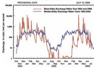
Comparison of daily discharges for water year 2005 and 2006 and period of record
