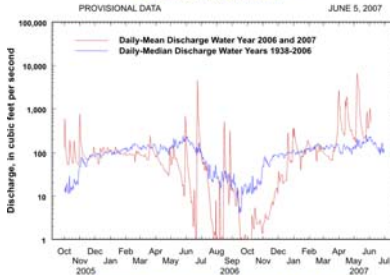
Comparison of daily discharges for water year 2006 and 2007 and period of record
