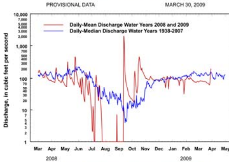
Comparison of daily discharges for water years 2008 and 2009 and period of record
