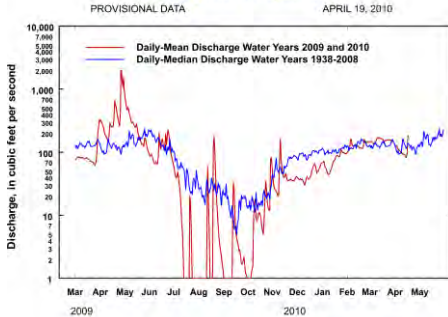
Comparison of daily discharges for water years 2009 and 2010 and period of record
